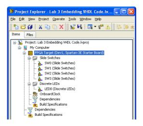
In this lab we are going to create a parity checker. We will put "LEDO" of the Spartan3E Starter board on when the input of the checker system (by use of "SWO", "SW1", "SW2" and "SW3") has even bits.
