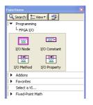
Place 2 I/O Nodes on the Block Diagram of the LabVIEW FPGA vi.
