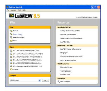
We have to create an Empty Project where we will add the Xilinx Spartan3E starter board on as a hardware target. In a future lab I will explain how we can create a HOST vi (this is a LabVIEW application that runs on a desktop PC) that communicates with a LabVIEW FPGA vi.
